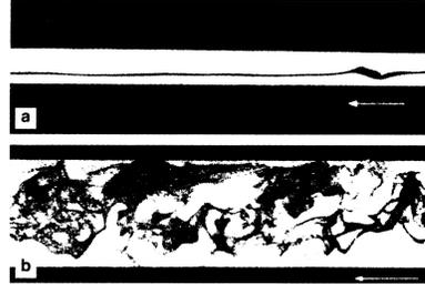
Figure 1.2: *Flow from right to left through a pipe: a) Laminar flow ( $Re = 1150$ ), b) turbulent flow ( $Re = 2520$ ). From (Schlichting, 1999) p. 13*
